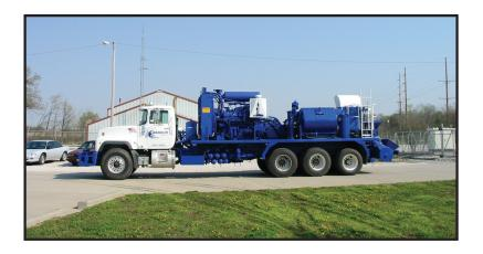
All of our fracturing units have densitometers, flow meters, pressure transducers installed on them, and these parameters are monitored throughout the job.
